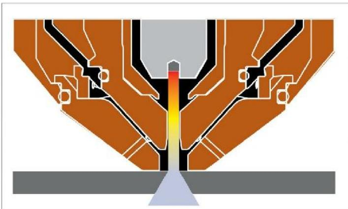
**Standoff, the distance between the workpiece and the tip of the torch, is critical to both cut quality and parts life.**
