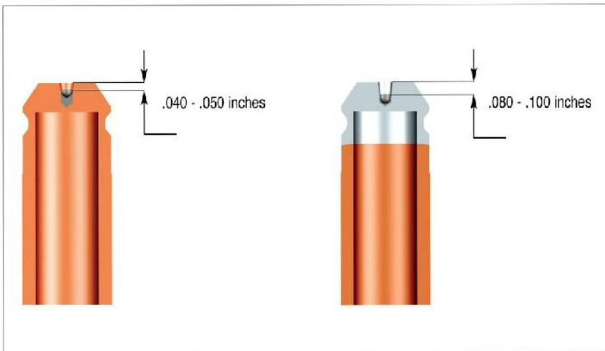
**Changing out consumables too soon or not soon enough are two common mistakes. The rules for when to change out electrodes is: Standard all-copper electrodes should be change when the hafnium pit depth is between 0.040 and 0.050 in., while silver tipped electrodes can reach a pit depth between 0.080 and 0.100 in.**
