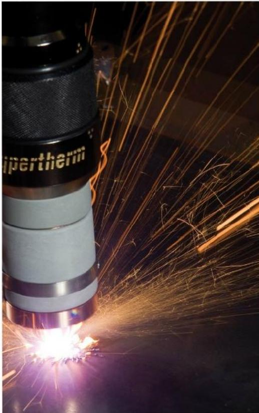
**Piercing too close to the plate is one of the biggest mistakes a plasma operator can make. Even one pierce too close can damage the torch and consumables.**
