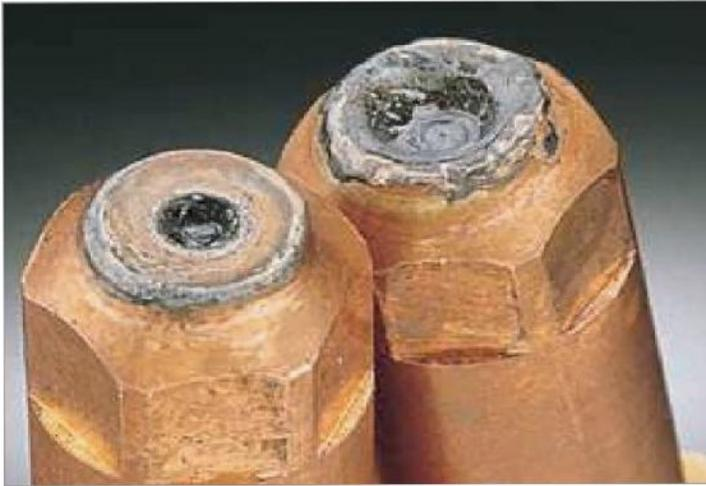
**The electrode on the left shows that it is about ready to be changed out. Compare to the electrode on the right, in which the hafnium is completely gone.**
